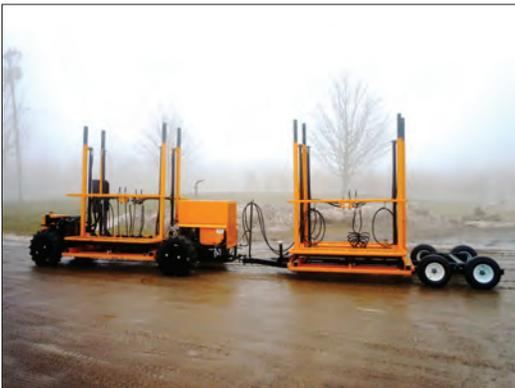
and picking. With auxiliary hydraulics, it is possible to use hydraulic pruners or run a hydraulically-driven air compressor with air pruners.
