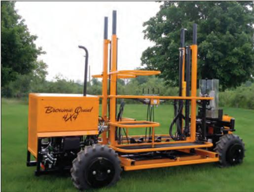
The Brownie Quad 4x4 is a self-propelled work platform with two individual platforms. These platforms have a working height that starts only 20" from the ground in the lowest
