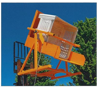
This view shows an optional anchor plate that can be used if no other chain attachment point is available.
