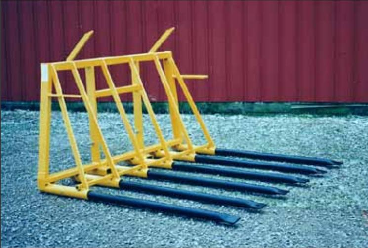
This heavy duty brush pusher is designed to float. It's tines are mounted under the frame and work like skis to follow the contour of your orchard floor. The easily replaceable tines are flattened on the ends and mounted close together to pick up smaller brush.
