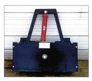
Rotator can be removed or reinstalled in minutes by one person.
