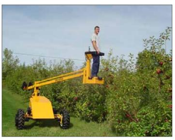
With years of proven dependability, the **New Brownie** has all three wheels powered by planetary drives. We have added larger wheels, wheel weights, and dual hydraulic pumps for smoother operation and cooler oil temperature.
